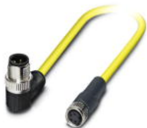
Sensor/actuator cable, 4-position, PVC, yellow, Plug angled M12 SPEEDCON, A-coded, on Socket straight M8, cable length: 0.5 m
