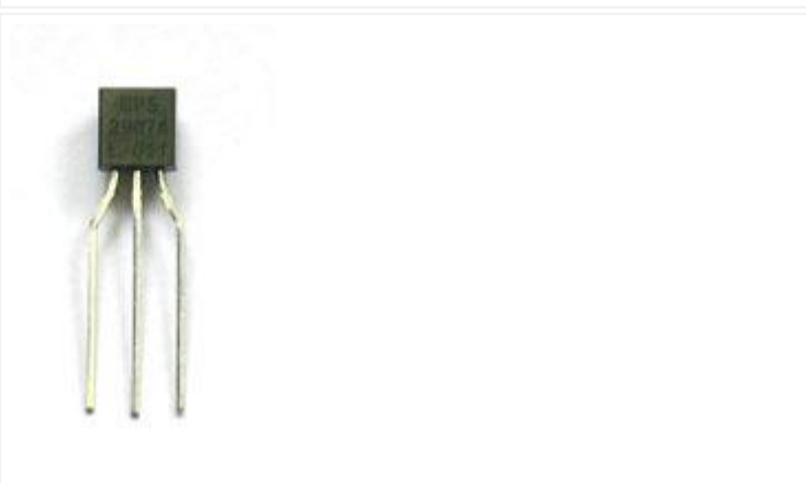
Q5 PNP transistor, EBC pinout Such as PN2907 or 2N3806 PN2907 1
