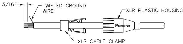
5. TWIST STRIPPED WHITE WIRES TOGETHER AND TIN. TWIST STRIPPED BLUE WIRES TOGETHER AND TIN. TWIST AND TIN GROUND WIRE.
