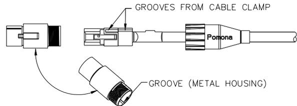
8. SLIDE PLASTIC HOUSING FORWARD AND THREAD ONTO METAL HOUSING AS SHOWN, PULL TEST 100 LBS MAX.
