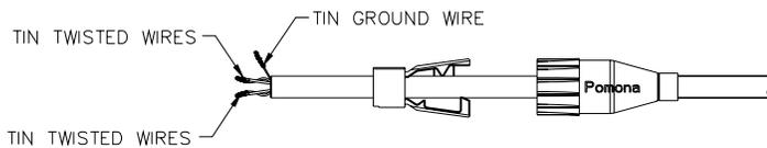
6. SOLDER GROUND WIRE TO THE NUMBER 1 CONTACT (CONTACT NUMBERS PRINTED ON PLASTIC HOUSING). SOLDER WHITE TWISTED PAIR TO NUMBER 2 CONTACT. SOLDER BLUE TWISTED PAIR TO NUMBER 3 CONTACT.
