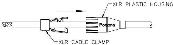
4. REMOVE BRAID AND FILLER EVEN WITH CABLE JACKET. SEPARATE GROUND FROM INNER WIRES AND TWIST. STRIP WHITE AND BLUE WIRES TO 3/16".
