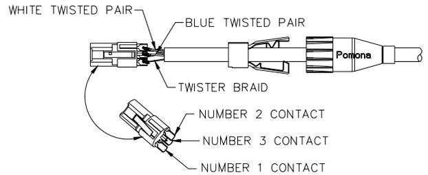
7. SLIDE CABLE CLAMP FORWARD OVER SOLDERED CONNECTION AND LINE UP THE KEYS (SLOTS) AS SHOWN. LINE UP GROOVES FROM CABLE CLAMP AND METAL HOUSING. SLIDE CABLE CLAMP ASSEMBLY INTO METAL HOUSING.
