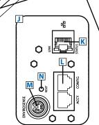
Network Interface: Connect to Ethernet for remote monitoring via SNMP, Web or Telnet. Add optional ENVIROSENSE accessory for temperature/humidity monitoring and dry contact interface.
