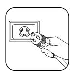
AC Input Connection: Insert L6-30P twist-lock plug into compatible L6-30R utility, generator or UPS outlet.
