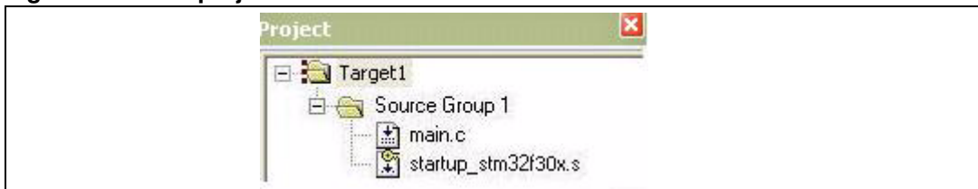
Figure 31. New project file tree structure
