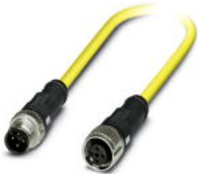
Sensor/Actuator cable, 4-position, TPE, yellow RAL 1021, Plug straight M12 SPEEDCON, A-coded, on Socket straight M12 SPEEDCON, A-coded, Cable length: 0.5 m
