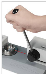
Ergonomic lever easily applies force and releases the sample.
