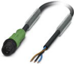
Sensor/Actuator cable, 3-position, PUR halogen-free, Black-gray RAL 7021, Plug straight M12, A-coded, on Free cable end, Cable length: 10 m, with plastic knurl
