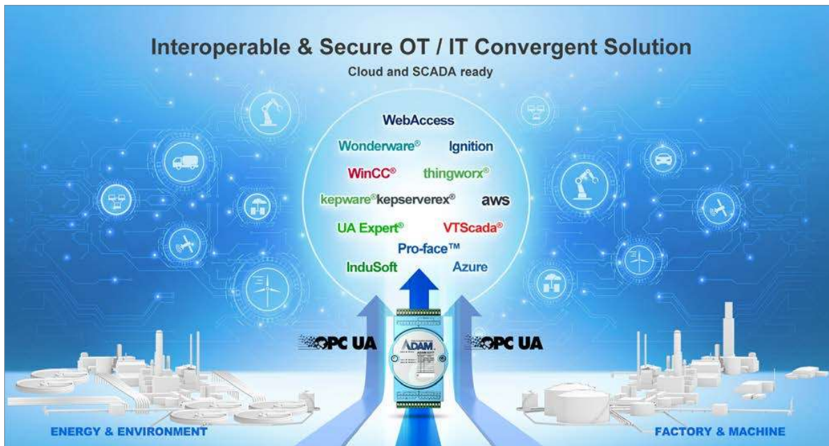
Figure 7: The Advantech ADAM-6300 series provides secure data transmission of I/O data to SCADA and cloud systems via the OPC UA Protocol.
