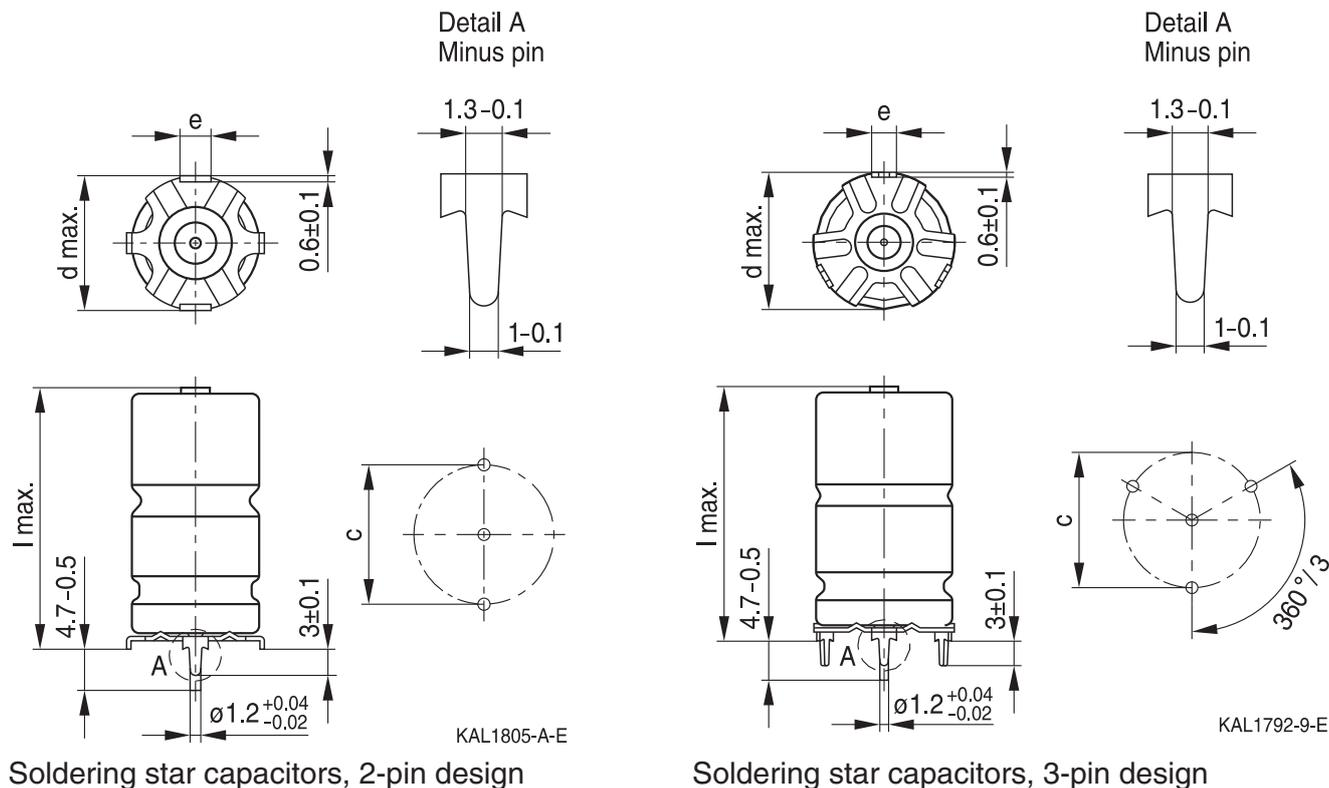
Soldering star capacitors, 2-pin design
