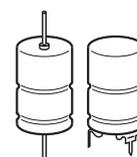
**B40700, Soldering star capacitors, version without sleeve**
