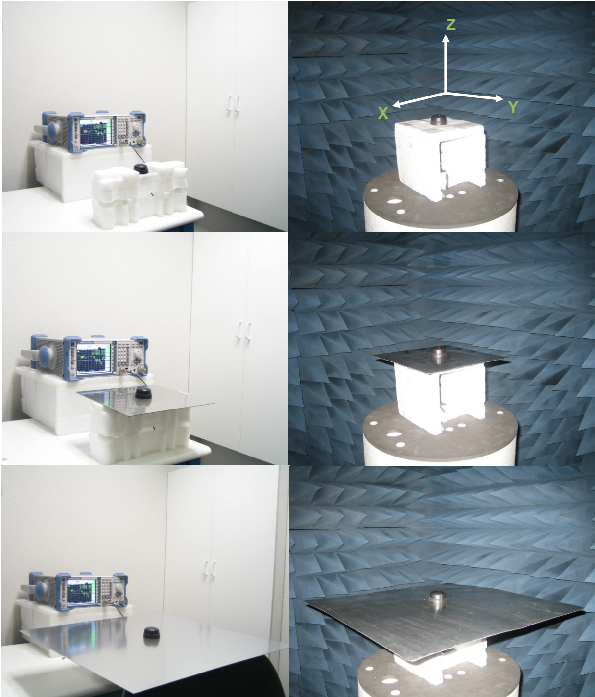
Figure 1. IS.04 Antenna test set up in free space, 30x30 cm metal plate and 60x60 cm metal plate, R&SZVL6 VNA (left) and R&S4100 CTIA 3D Chamber (Right).
