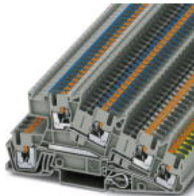
Installation ground terminal block, Push-in connection, cross section: 0.14 mm 2 - 4 mm 2 , AWG: 26 - 12, width: 5.2 mm, color: gray, mounting type: NS 35/7,5, NS 35/15
