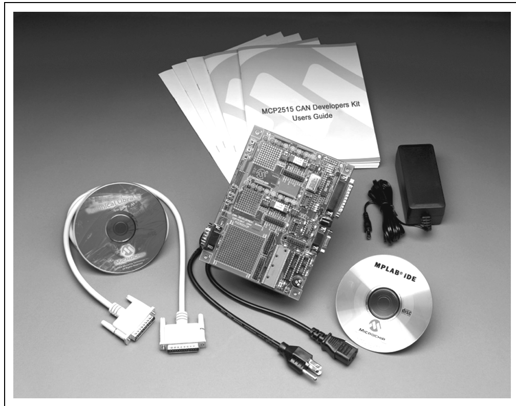
FIGURE 2-1: MCP2515 DEVELOPMENT KIT COMPONENTS
