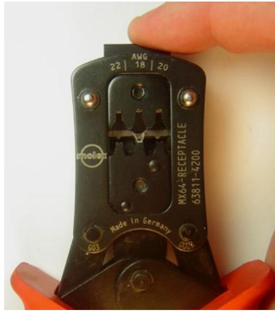
2.) Insert the correct terminal and press the wire-stop down.
