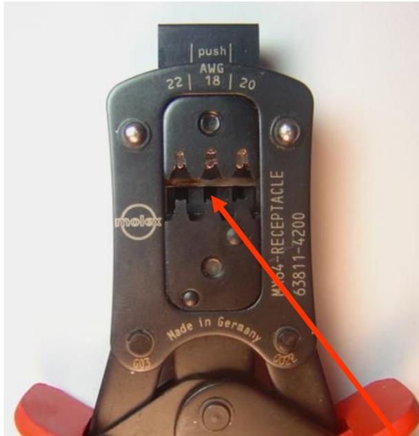
1.) Identify the wire gauge you need to crimp. Notice the rectangular shape of the terminal cavity.
