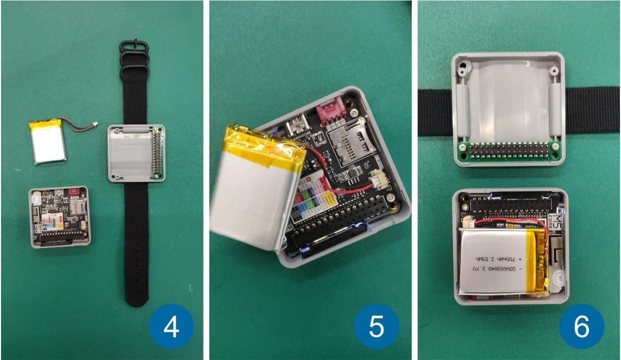
Installation base: According to the position of the BUS bus on the main unit, the watch base is vertically inserted into the main unit and locked with the matching screws to complete the assembly.
