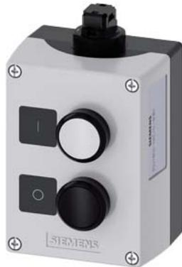
AS-Interface enclosure for command devices, 22 mm, round, Enclosure material plastic, enclosure top part gray, 2 control points plastic, Recess for labels, B=Pushbutton white, label: I, 1 NO, spring-type terminal, A=Pushbutton black label: O 1 NC, spring-type terminal, floor mounting, Insulation displacement system on top, Labels enclosed
