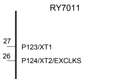
Figure 6 – 5 Connection of the XT1 and XT2/EXCLKS Pins When an On-Chip Oscillator Is in Use Note
