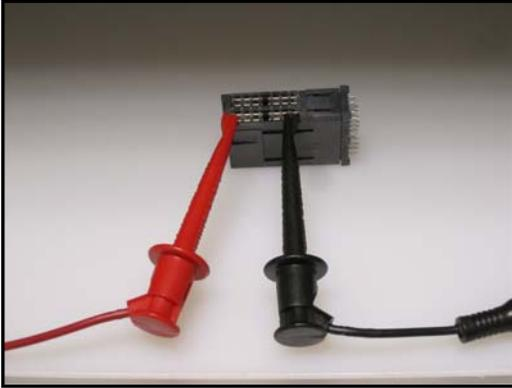
Figure 4- Front to Back Withstand Voltage test setup
