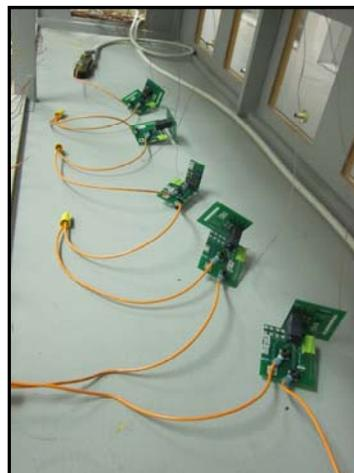
Figure 6- Temperature Rise vs. Current test setup
