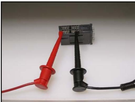
Figure 2- Front to Back IR test setup
