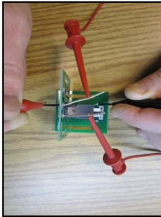
Figure 1- Low Level Contact Resistance test setup
