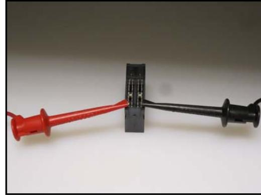
Figure 5- Left to Right Withstand Voltage Test setup
