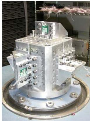
Figure 7- Vibration/Shock Setup
