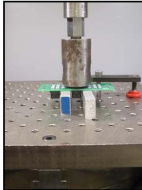
Figure 12- Typical Compliant Pin push-out force test setup.
