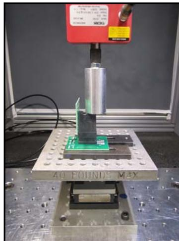
Figure 9- Mating Force Test Setup
