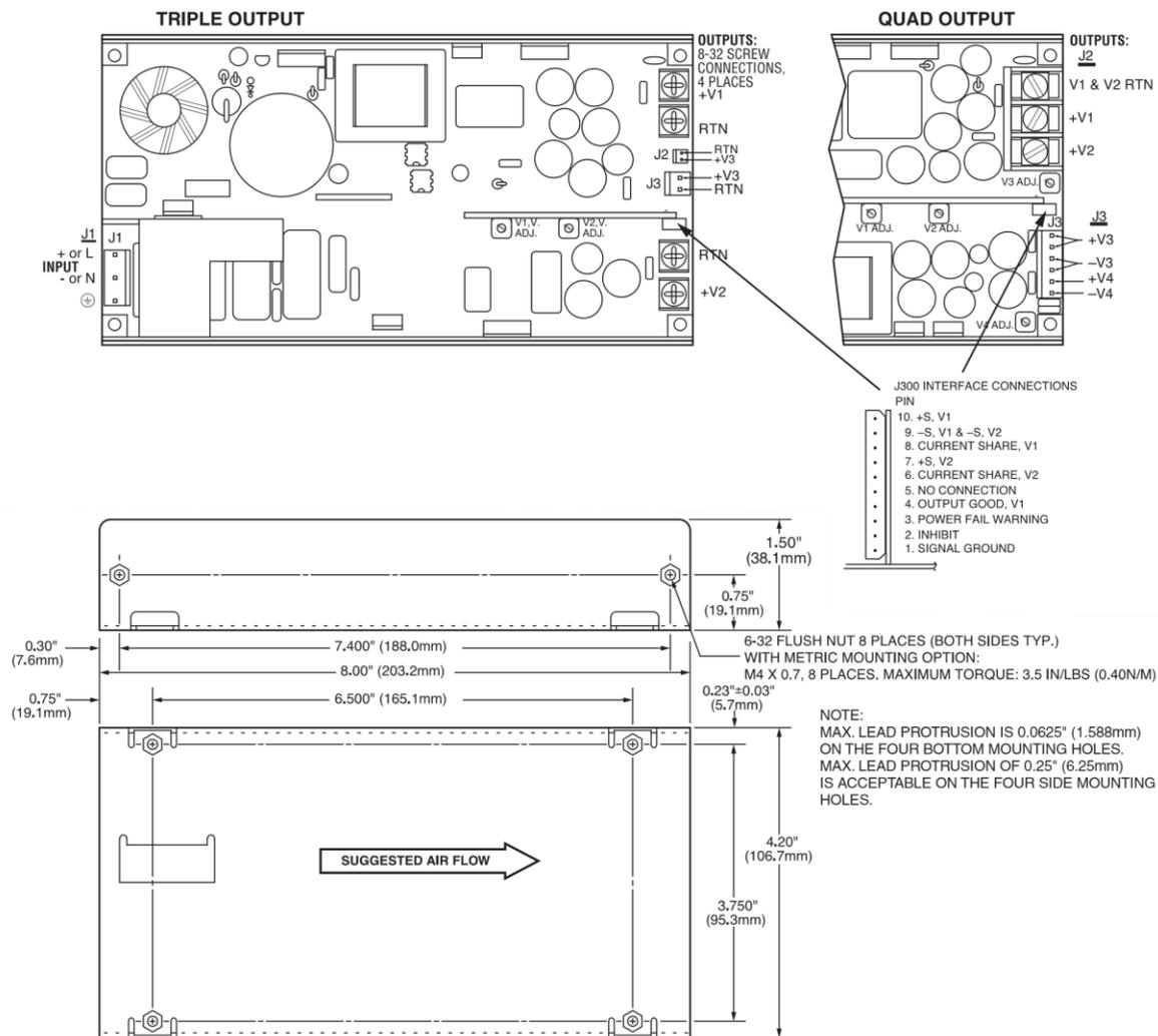
Figure 2. Mechanical Drawing – Triple & Quad Output
