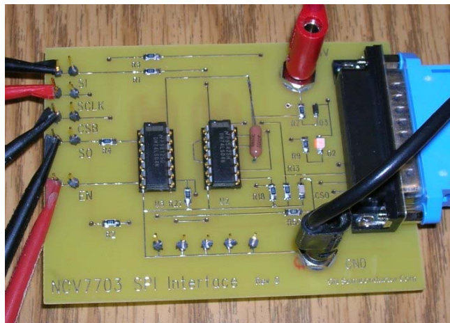
Figure 2. NCV7703 SPI Interface Buffer Board
