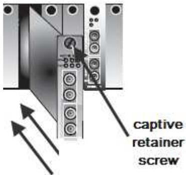
**All open slots in the chassis must be covered with a face plate in order to maintain proper circulation throughout the chassis**
