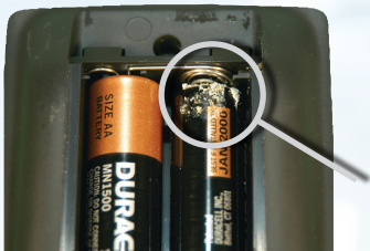
Corrosion you CAN see
