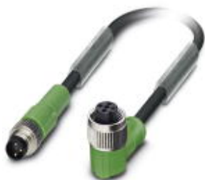
Sensor/actuator cable, 3-position, Variable cable type, Plug straight M8, on Socket angled M12, A-coded, cable length: Free input (0.2 ... 40.0 m)
