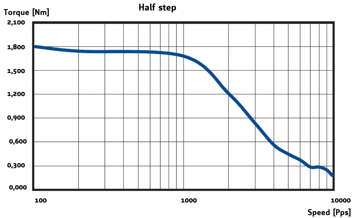
Figure 5.4: QSH5718-76-28-189 speed vs. torque characteristics
