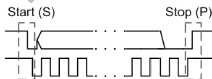
Figure 8.1: 2-Wire serial interface Start / Stop condition
