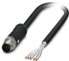
Sensor/Actuator cable, 5-position, PE-X halogen-free, black, shielded, Plug straight M12 SPEEDCON, A-coded, on free cable end, Cable length: 10 m, For railway applications
