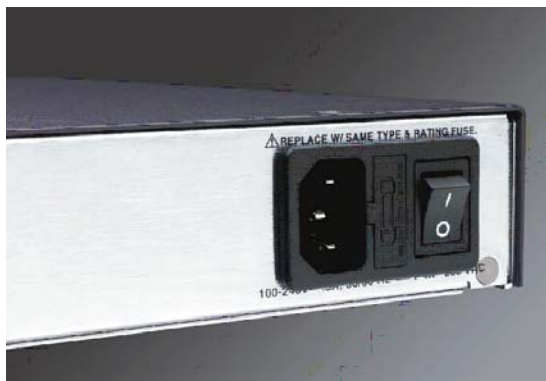
Figure 3-4 AC Power Input and Power Switch (SLCxxxx2N)
