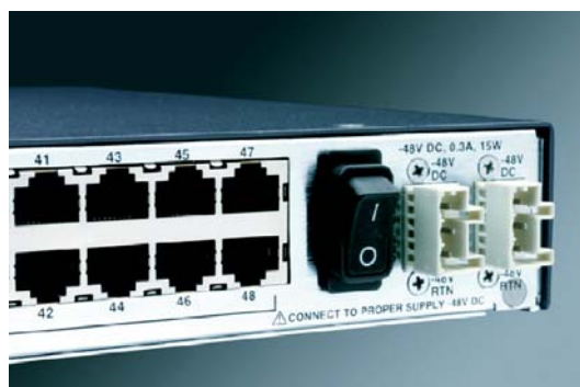
Figure 3-5 DC Power Inputs and Power Switch (SLCxxx24T)
