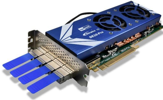
Figure 9-2 QSFP28 Transceiver Loopback Test in Progress
