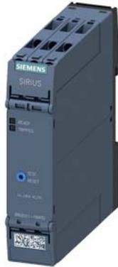
Thermistor motor protection relay Standard evaluation unit 22.5 mm enclosure screw terminal 2 change-over contacts US = 24 V-240 V AC/DC Manu/Remote-Reset with ATEX approval 2 LEDs (READY/TRIPPED) galvanic isolation Test/reset button Wire break monitoring Short circuit monitoring
