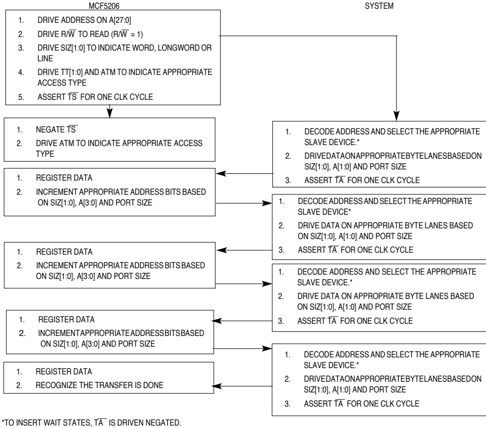
Figure 6-8. Bursting Word-, Longword-, and Line-Read Transfer Flowchart
