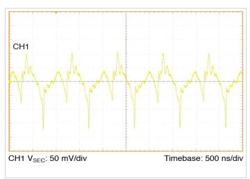
**Figure 11** — Full load ripple, 10 µF C<sub>PRI\_IN\_EXT</sub>; No external C<sub>SEC\_OUT\_EXT</sub>. Board mounted module, scope setting : 20 MHz analog BW
