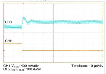
**Figure 13** — 125 A – 0 A transient response:  $C_{PRI\ IN\_EXT} = 10\ \mu\text{F}$ , no external  $C_{SEC\_OUT\_EXT}$
