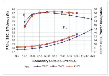
**Figure 8** — Efficiency and power dissipation at  $T_{CASE} = 90^{\circ}C$
