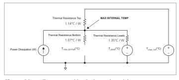
Figure 20 — Top case and leads thermal model
