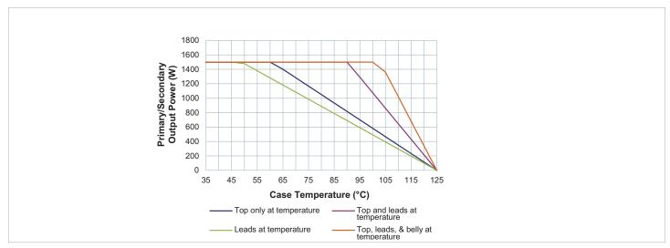
Figure 1 — Specified thermal operating area
