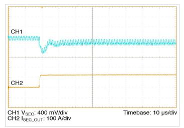
**Figure 12** — 0 A– 125 A transient response:  $C_{PRI\_IN\_EXT} = 10 \ \mu\text{F}$ , no external  $C_{SEC\_OUT\_EXT}$
