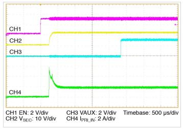
**Figure 15** — Start up from application of EN with pre-applied  $V_{PRI\_DC} = 384 \text{ V}$ , 50%  $I_{SEC\_DG}$ , 100%  $C_{SEC\_OUT\_EXT}$
