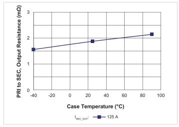
Figure 9 —  $R_{SEC}$  vs. temperature; Nominal  $V_{PRI\_DC}$  $I_{SEC\ DC} = 100\ A$  at  $T_{CASE} = 90^{\circ}C$
