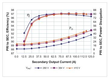
**Figure 6** — Efficiency and power dissipation at  $T_{CASF} = -40$ °C
