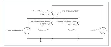
Figure 21 — Top case thermal model
